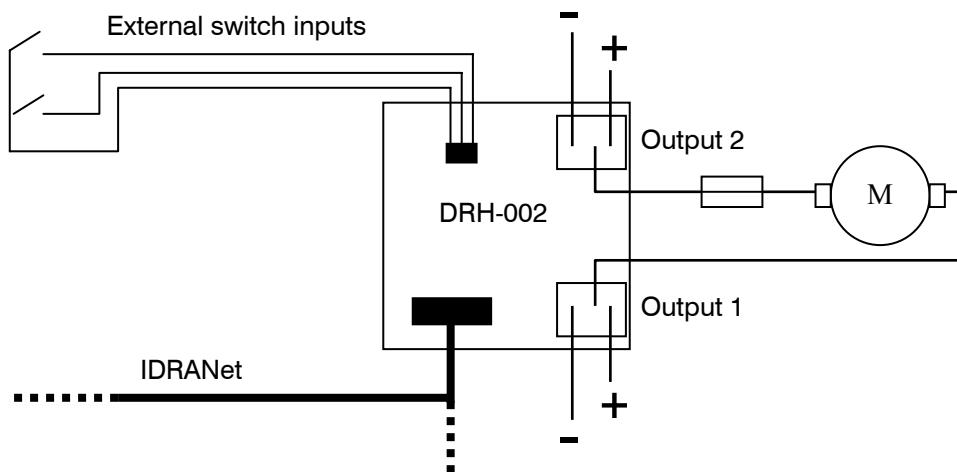
Note: Though both digital and analogue filtering are employed on all inputs, for longer (eg. >3m) normally open input connections it is advisable to take additional noise protection precautions, eg.: Use twisted pair or shielded cables (one side/shield to 0V).
