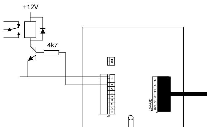
Note: On module power up, despite any user defined initialisation state, outputs will at least momentarily rise to 3.3V. So in this example the relay will be at least briefly energised after a power up. This logic can be inverted, for example, by using two NPN transistors instead of one
