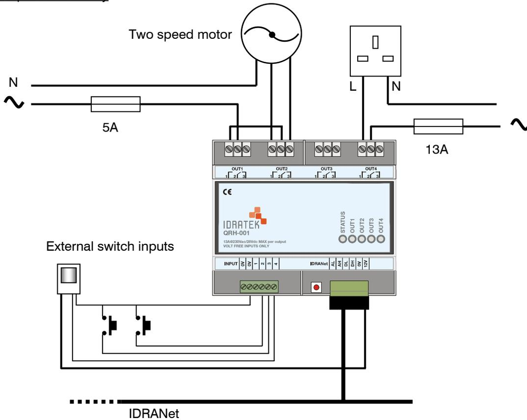
Note: The QRH-001 module does not incorporate internal fuses. External fuses or circuit breakers should be fitted to suit the application and module maximum current capacity should not be exceeded
