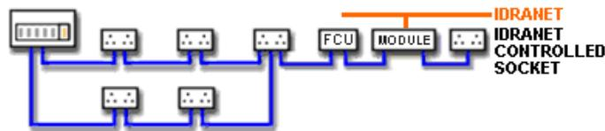
The cable from the back of the ring socket to the FCU must be suitably rated, i.e. at least 32A (4mm<sup>2</sup>). A short circuit fault in this piece of cable could deliver 16A from each direction of the ring up to the maximum current for that circuit (set by the MCB probably to 32A).
