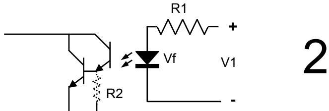
Darlington pair configuration in 2 gives much higher sensitivity but there is a small risk that the 'on' voltage drop across the output (~0.7-0.8V) may not be low enough for the digital input to register zero for all IDRATEK modules\*. Depending on application R2 may be required to improve switch off speed. Typical transistor BC550C and, if used, R2 might be ~10k
