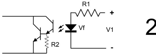
Darlington pair configuration in 2 gives much higher sensitivity but there is a small risk that the 'on' voltage drop across the output (~0.7-0.8V) may not be low enough for the digital input to register zero for all IDRATEK modules\*. Depending on application R2 may be required to improve switch off speed. Typical transistor BC550C and, if used, R2 might be ~10k
