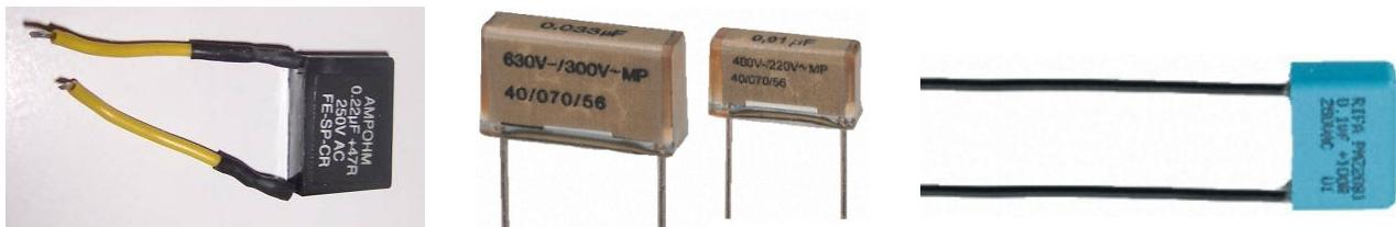
It is best to fit suppressors at the load side rather than at the relay terminals:
