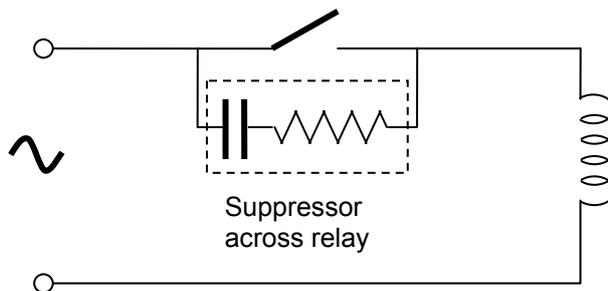
However it should be noted that a capacitive suppressor connected across a relay terminal (rather than load) will allow a small leakage current to flow to the load even when the relay contacts are open.
