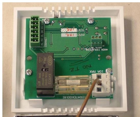
The return from the SRH relay normally open connection (NO) is then connected to the mains socket outlet. Again this cable must be rated at 32A (4mm<sup>2</sup>).
